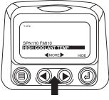
4. To acknowledge and "Hide" the fault and return to the single or four parameter display touch the "Enter Button".
